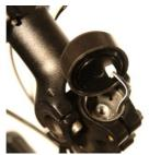
•Fasten the Cycle2Charge with the delivered screw.
